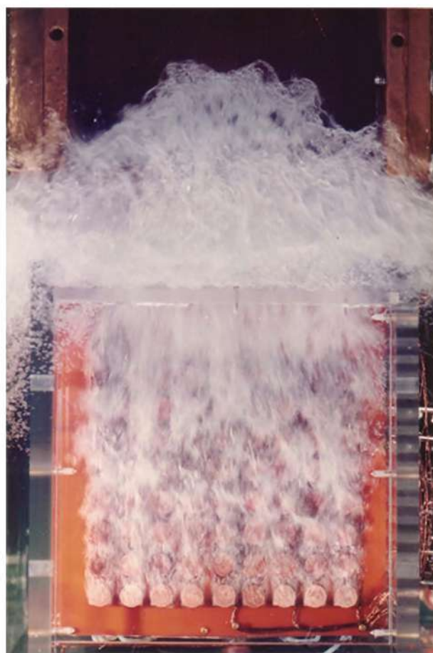
Fig. 11 – Boiling cooling of simulated chips in the 1980s. 88
